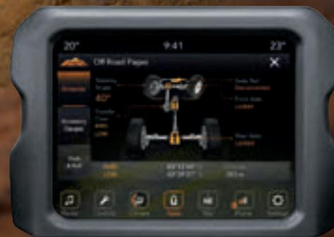
**OFF-ROAD PAGES** Access real-time performance data like suspension travel or keep an eye on your tilt and pitch. In-depth vehicle diagnostics, including wheel turn, articulation and transmission temperature, all help to provide an optimized experience. Available.
