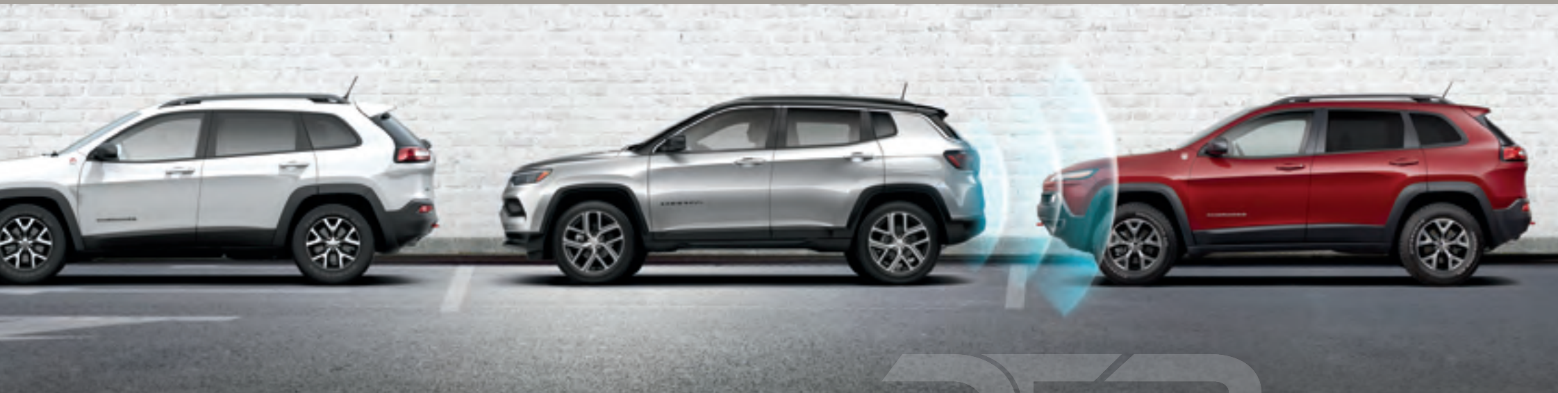
PARALLEL AND PERPENDICULAR PARK AND UNPARK ASSIST SYSTEM 15 This active guidance system controls steering automatically. You can take your hands off the steering wheel and let the system's ultrasonic sensors help you ease into parking spots as you gently brake and change from Reverse to Drive as needed. Unpark Assist 15 helps you navigate your way out of parking spots. It controls the vehicle's steering while providing the driver with gear and braking instructions. Available.
