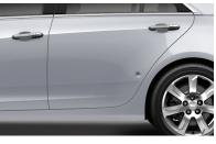
Fewer than four dings or dents less than 2.5cm in diameter per panel that have not penetrated or cracked the paint surface.
