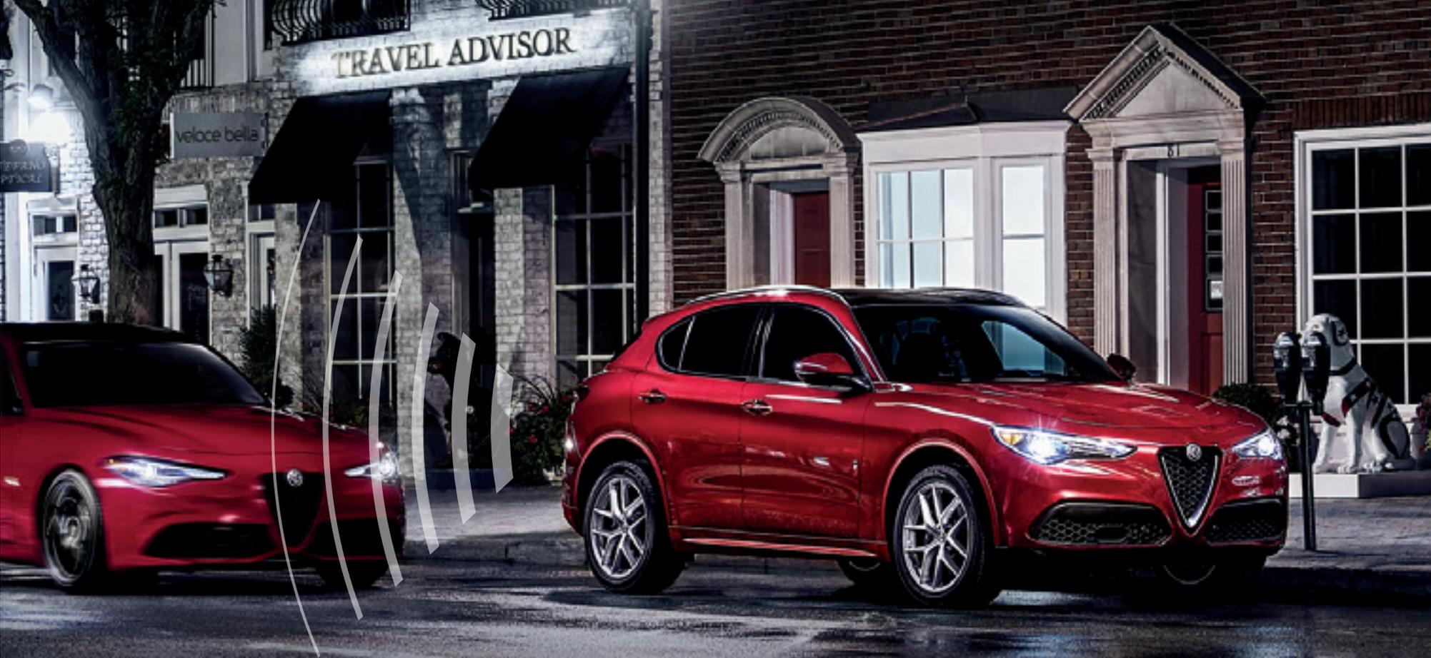
**ACTIVE BLIND-SPOT / "SIDE ASSIST"**<sup>2</sup> Change lanes confidently or stay right where you are with this warning system that detects approaching traffic from behind, along with its rate of travel. An LED signal in the corresponding exterior side mirror indicates a vehicle that's too close, while steering-wheel resistance adds another accident-avoidance action. Available.
